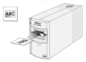
To scan a film strip with the SA-20 strip-film adapter, grasp the film lightly by both edges and slide it into the film slot a short distance. The adapter's feed mechanism will be activated and the film will be fed into the scanner automatically.
