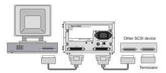
3. Confirm that the last device in the chain is terminated
