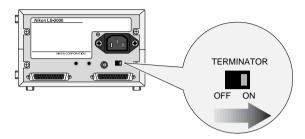
2. Connect the SCSI cable to either of the two SCSI connectors on the rear of the scanner and connect the other end to the next device in the chain
