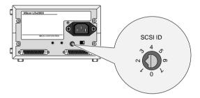
When choosing another ID for the scanner, bear in mind that the computer will usually have an ID of either "0" or "7," and that internal hard disks often have IDs of "0" or "1." In the case of Macintosh computers, the computer will have an ID of "7," while the internal hard disk and CD-ROM drive often have IDs of "0" and "3," respectively. In general, it is recommended that you set the scanner's ID to any number other than zero, one, three, and seven that is not used by another SCSI device.
