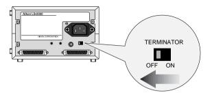
2. Connect the SCSI cable from one of the devices in the chain to either of the connectors on the rear of the scanner, then connect a cable to the remaining connector and attach the other end to a connector on the next device in the chain
